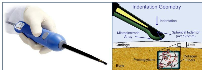
The Arthro-BST is an arthroscopic device that directly measures cartilage **streaming potentials** by compressing cartilage with a spherical indenter containing an array of 37 gold microelectrodes ( $r=3.2$  mm, 5 microelectrodes/mm<sup>2</sup>).
