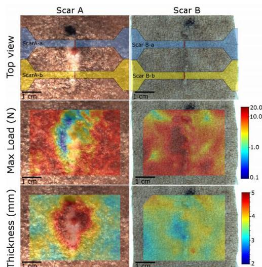
Figure 2. Photodocumentation of the excised strips (tensile test) on each sample and mappings of the maximum load and thickness obtained through the novel indentation technique.
