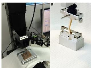
Figure 1. A) Experimental set up of a skin sample on the multi-axial mechanical tester for indentation; B) Experimental set up of an excised strip on a uniaxial mechanical tester for tensile test.
