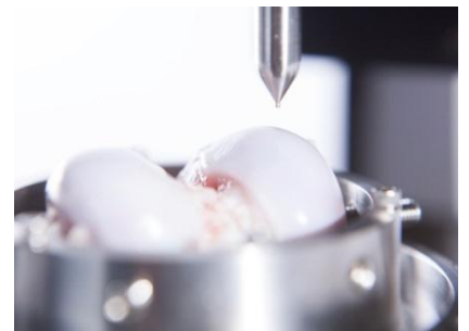
Ovine (sheep) condyles installed under a spherical indenter (d=1 mm) for normal indentation mapping
